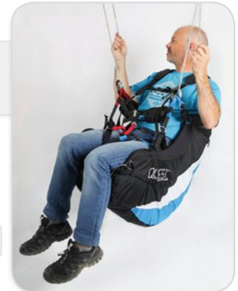
Before your first flight, we recommend to suspend the harness from a suitably strong point to check that it fits you correctly and to become familiar with the features and adjustments. You can set the shoulder adjustment-straps to find the best fit, and adjust the lumbar support so that they leave you in a comfortably reclined position. Only ever suspend from carabiners attached to the main hang points.
