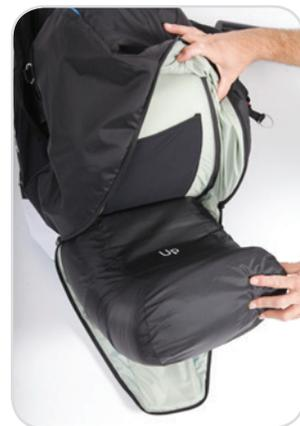
To install the under seat protection, open the lower zipped compartment found within the rear pocket. The protector is clearly marked 'up' and 'front' so that you can orientate it properly. Close the zipped compartment once the protector is in place.
