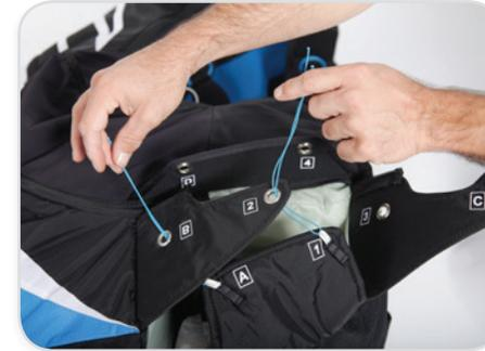
To close the flaps, use suitable pieces of magic string or plastic and pull the white loops (A and 1) through eyelets B and 2, then C and 3.
