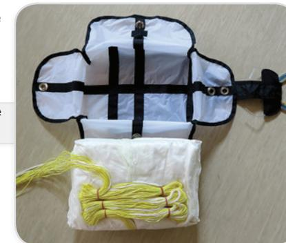
Insert the parachute into the deployment bag and secure the deployment bag with the lines in the normal way. Depending on the size of your parachute you can use any of the eyelets for the best fit.
