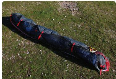
**Step 9.** Turn the Saucisse on its side and make the first fold just after the LE reinforcements. Do not fold the plastic reinforcements, use 3 or 4 folds around the LE.
